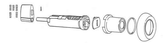
The subject lock is a standard assembly incorporating new parts; primarily the lock cylinder and the pawl.
