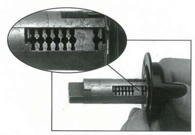
Some GM ignition locks are supplied with the 2/3 tumbler positions filled. This is not a defect.
